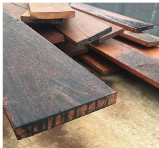
**Photograph 2 - Mould stains on linseed oiled decking**
